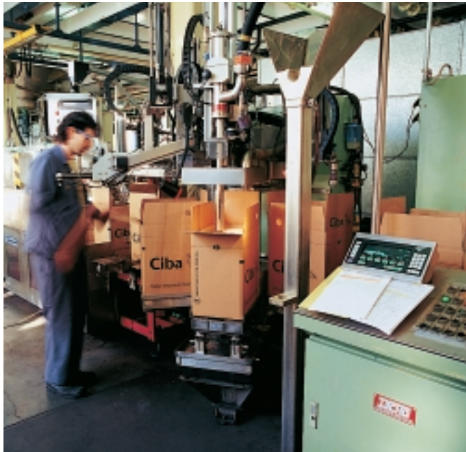
"Bag in box" below level filling
