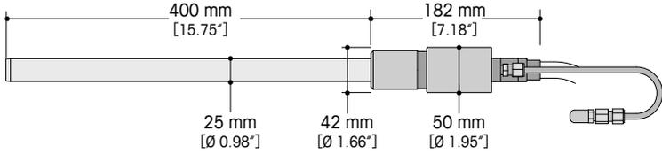
**Figure 2.** Probe dimensions—G600R
