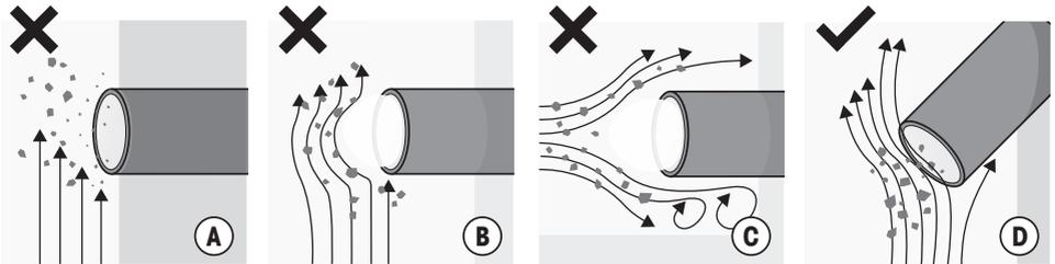
**Figure 5.** Implementation of a ParticleTrack instrument: (A) flush with wall of vessel or pipeline; (B) inserted tangentially to process flow; (C) inserted perpendicular to process flow at an elbow; and (D) inserted at optimal angle (45°) relative to process flow.
