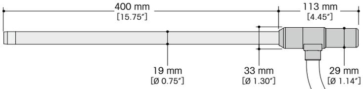
**Figure 4.** Probe dimensions—G600B
