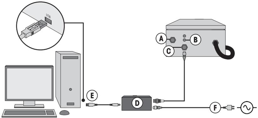
**Figure 6.** Instrument connections: (A) Power; (B) Air inlet for probe scanner; (C) Fiber communication connection; (D) Fiber-to-USB extender; (E) USB cable; (F) Extender power supply
