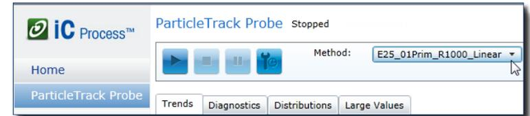
2. Select the Method to use for the particle or droplet system according to your SOP. After method selection, the Start icon button becomes enabled.
